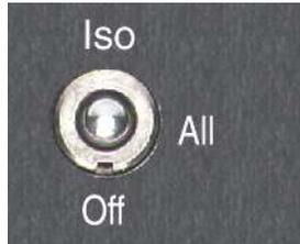
**ISO:** (Up Position): The pilot is isolated from the intercom and is connected only to the aircraft radio. He will hear the aircraft radio reception (and sidetone during radio transmissions if provided by the transceiver). Copilot and passengers will hear the intercom and music on Entertainment input, but not the aircraft radio receptions or pilot transmissions.
