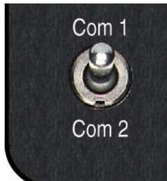
The PMA4000-Series has an automatic selector mode. Audio from the selected transceiver is automatically heard in the headsets and speaker (when selected). You can check this function by switching from COM 1 to COM 2 and watch the selected audio light on the selector change from C1 to C2. This ensures the pilot will never transmit on a radio is not listening to.
